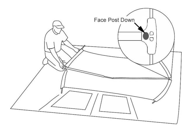
5) Match the ends of the T-poles so that they are touching. Grasp both poles firmly and push down.
